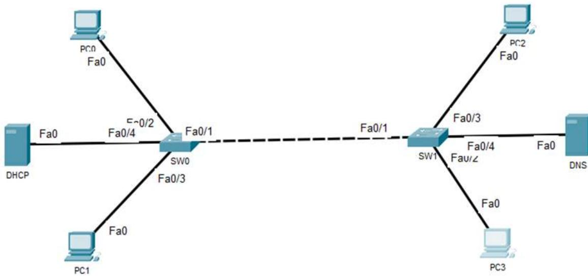
Use the following address block (192.168.9.0 255.255.255.0) to configure the network above. The network status is initial, no configuration has yet been carried out.
