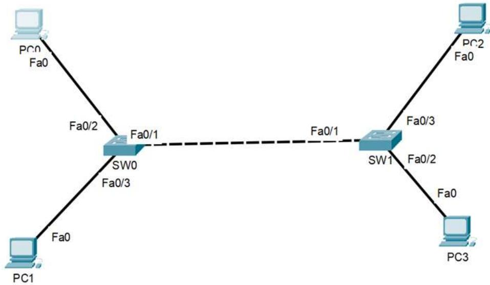
The above network has the address 172.24.224.0/19. We are in an initial state, there has not yet been any network communication, all the ARP tables are empty.
