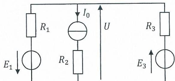
b.  $U = \frac{\frac{E_1}{R_1} + I_0 - \frac{E_3}{R_3}}{\frac{1}{R_1} + \frac{1}{R_2} + \frac{1}{R_3}}$
