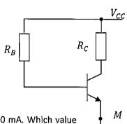
1. We want to tune the current in the resistance  $R_{\it C}$  to a value of 100 mA. Which value of  $R_{\it B}$  must be chosen?
