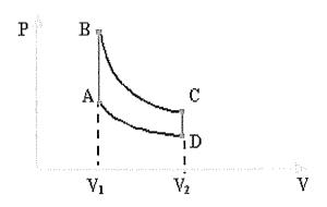
The transformations DA and BC are adiabatic whereas the transformations CD and AB isochoric. Oen defines  $a = V_2 / V_1$  the ratio between volumes (called the compression rate). Remember that the molar capacity  $\mathbf{c}_v$  is constant during this cycle.
